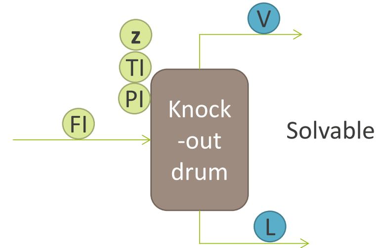
Additional measurements (temperature, pressure and composition) and VLE relationships allow estimating unmeasured streams
